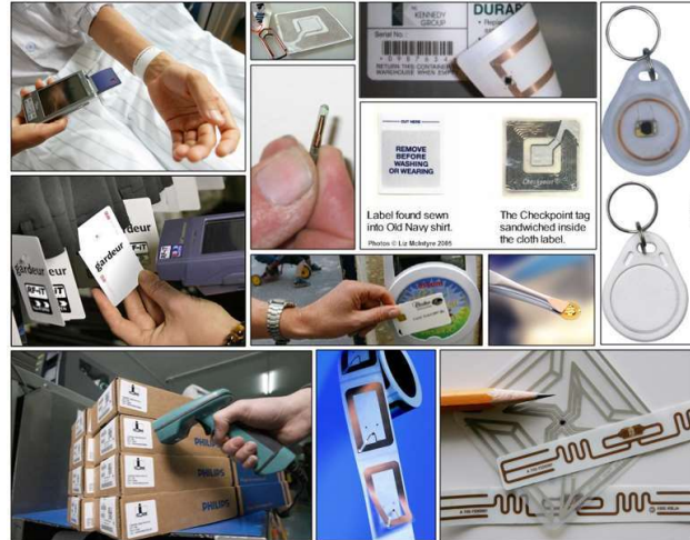
Figure 7: Various form factors and uses of RFIDs; readers are also shown in some of the images
