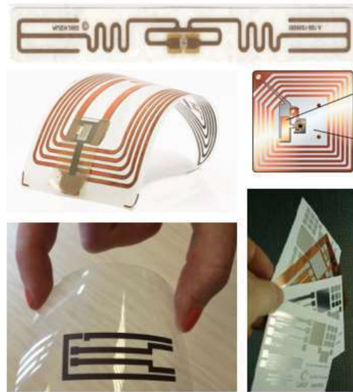
Figure 39: Examples of flexible, printed antennas used for RF applications
