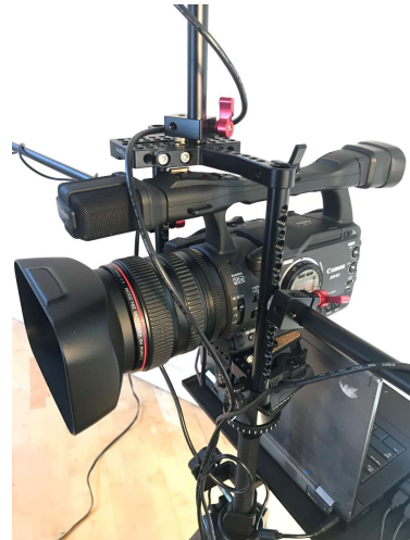
Figure 20: Close up of the camera inside the cage, clamps are used to attach the rods, and ultimately the anchor boards to the rig, creating a single unit that moves in unison
