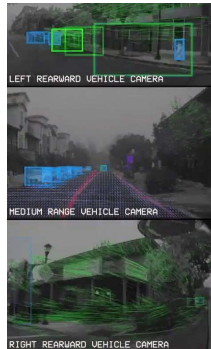
Figure 2: Example's Tesla's computer vision system which can detect lanes, road boundaries in-path objects, road lights, road signs, and other objects.
